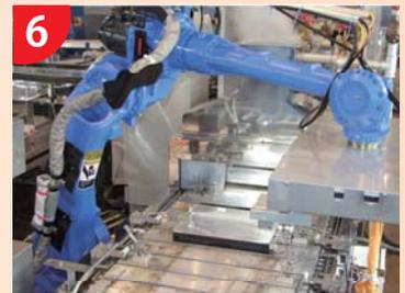
6 Opening molds by handling robot
