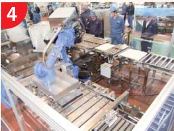
4 Carrying molds to steamer by handling robot
