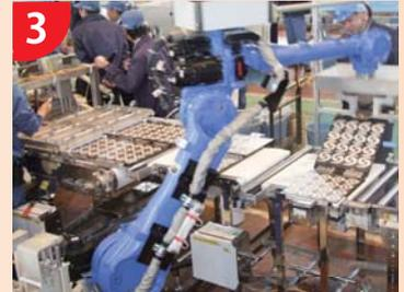
3 Folding molds by handling robot
