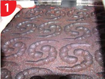
1 Coloring by spraying on molds
