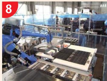
8 Carrying molds to washing C/V by handling robot
